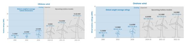
Figure 7 The average size of offshore wind turbines grew by a factor of 3.4 in less than two decades and is expected to grow to output capacity of 15–20 MW by 2030 while the size of onshore wind turbine is expected to grow by more than 5 times over the last 2 decades<sup>22</sup>
