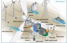
Figure 8 Inside of a wind turbine and ecosystem of onshore wind<sup>23</sup>
