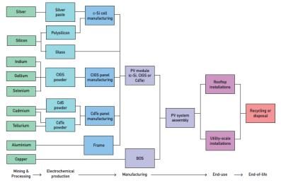
Figure 14 Overview of a solar PV supply chain<sup>28</sup>
