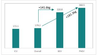
Figure 22 Average Aluminium Content per vehicle - Comparison by Powertrain Variant (Net weight in kg)<sup>46</sup>
